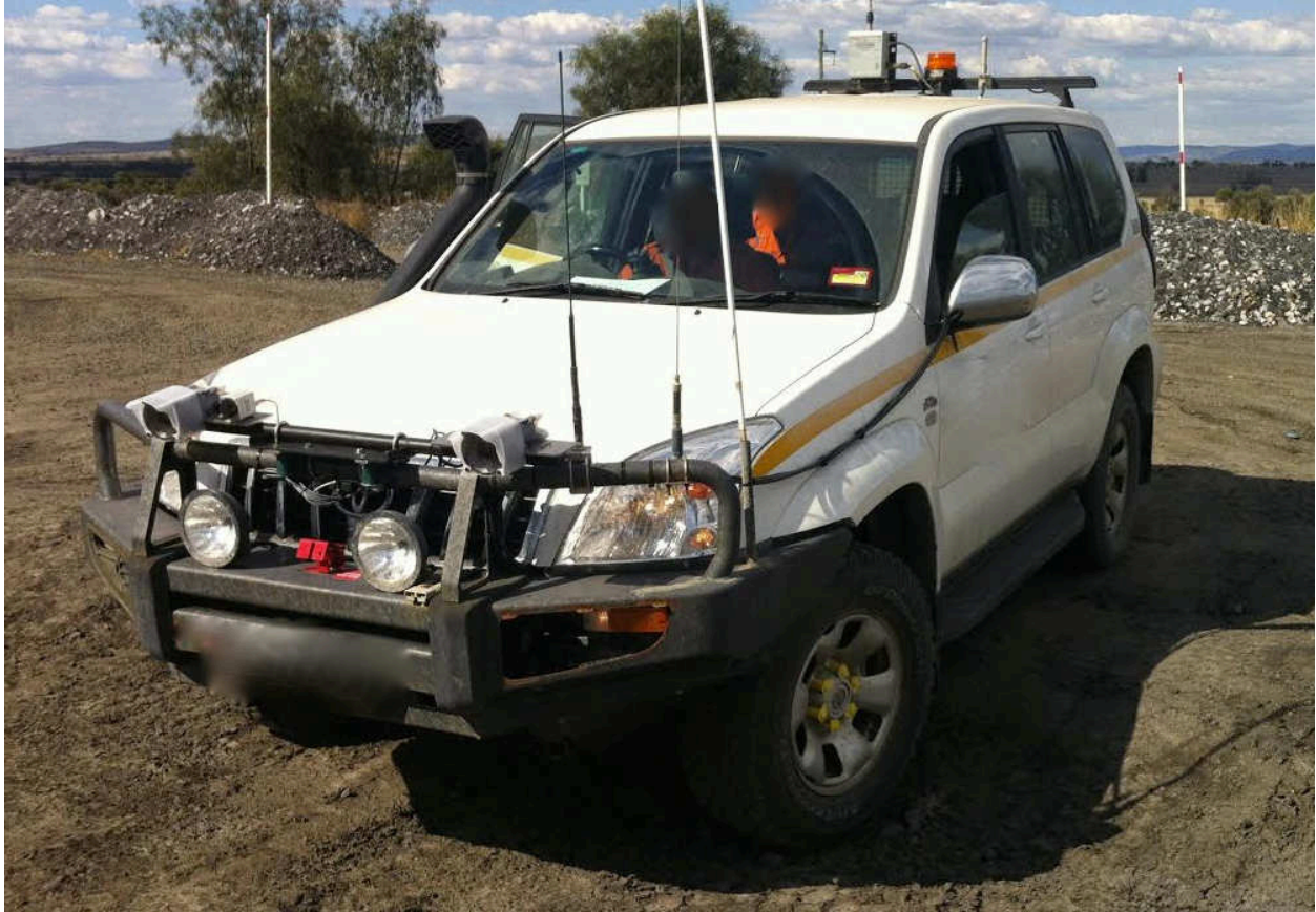
Figure 10: The experimental dataset gathering vehicle with cameras mounted to the bullbar. Note: all images used in this paper were captured from the camera on the left hand side of the vehicle.
